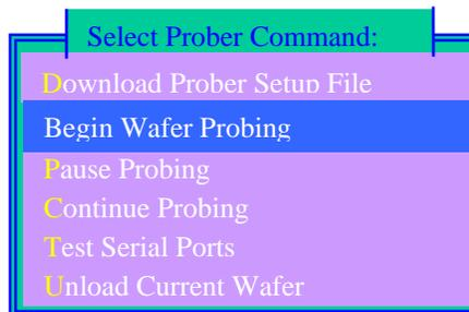
As the lot is testing, every 5<sup>th</sup> wafer must receive and pass a microscope inspection before the next 5 wafers can be tested. The purpose of the inspection is to insure that the setup is still good and that no drifting, mis-stepping, or probe damage has occurred.
