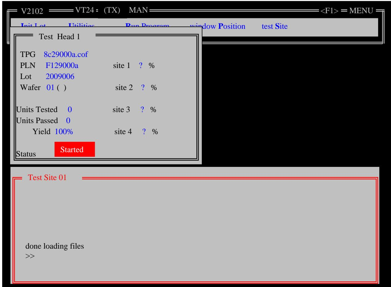
On this same screen, verify that the plan file (i.e. "PLN" in the "Test Head 1" box above) is correct for the device being run.
